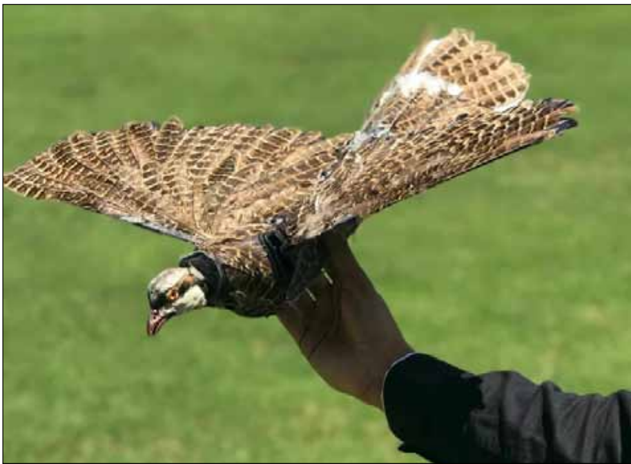
A taxidermied bird is equipped with a drone to simulate actual bird flight.
